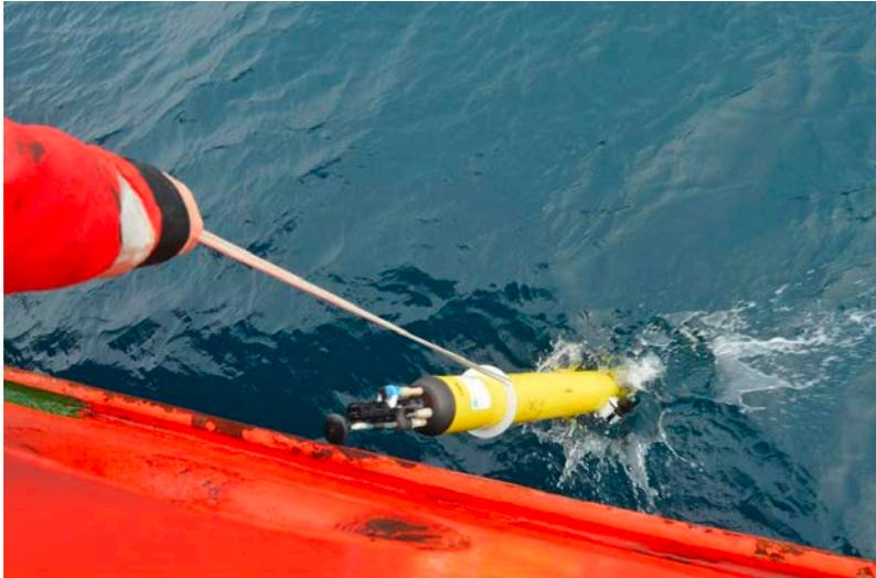
These deployments can only be done at slow ship speed and on the lee side of the vessel. We will aim for these deployments to occur at low ship speed just as we leave a CTD station.
