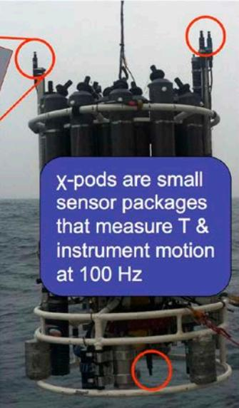
$\chi$ -pods are small sensor packages that measure T & instrument motion at 100 Hz
